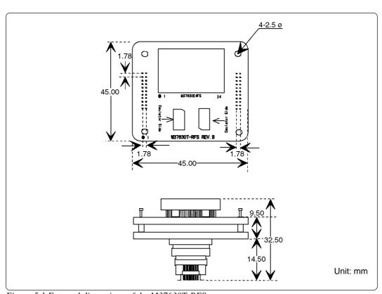
Figure 5.1 External dimensions of the M37630T-RFS
